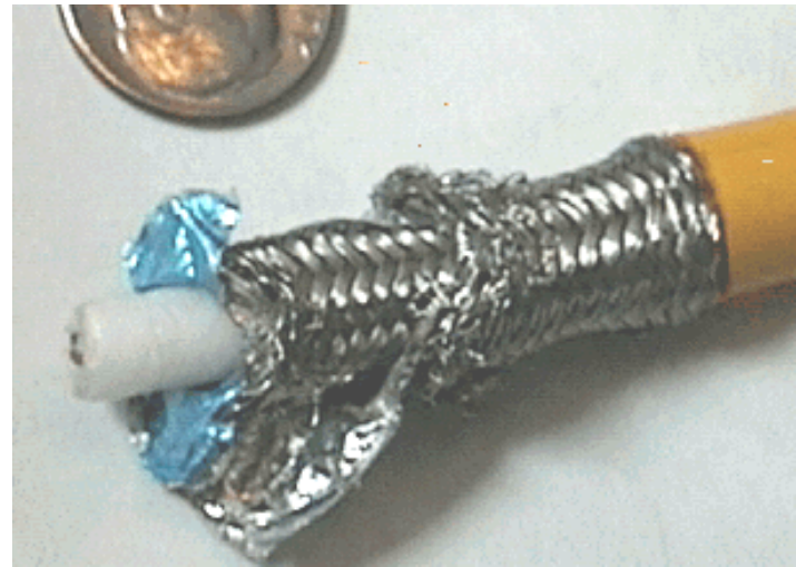
Thick ethernet - 10Base5
